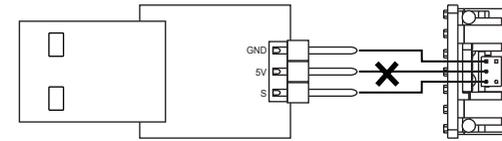
**Never connect the 5V output from USB adapter to ESC, or ESC will not work normally.**
