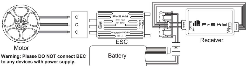
**Warning: Please DO NOT connect BEC to any devices with power supply.**
